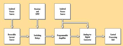
Figure 2. Measurement processing operations.
