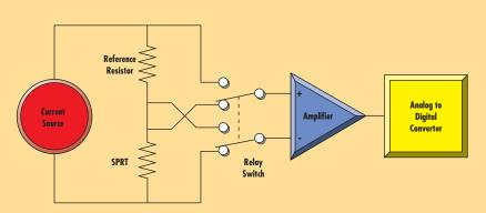
Figure 1. Simplified schematic diagram of the measurement circuit.
