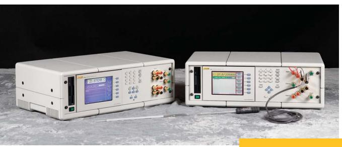
Fluke Corporation Hart Scientific Division's Super-Thermometers are recognized in metrology laboratories around the world for their ease of use and reliable accuracy. The Model 1575A Super-Thermometer is accurate to 0.001°C or 4ppm. The Model 1590 Super-Thermometer II is accurate to 0.00025°C, or 1 ppm.
